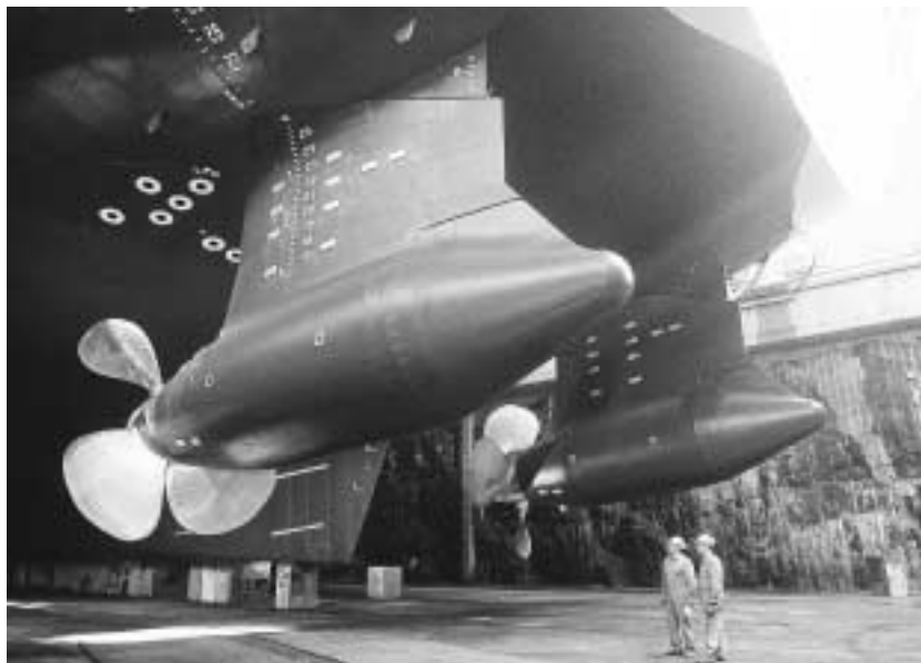
Fig. A9. The Azipod (Azimuthing Podded Drive) was conceived to give ships more manoeuvrability, with a motor inside a submerged pod that is 360 degrees' steerable (photograph courtesy of ABB).
